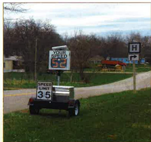
The ValuPro 2012 speed trailer is designed to help communities control speeds at a designated site while simultaneously collecting data related to average speed and vehicle volume.
